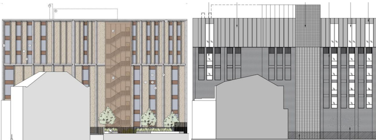
Images 12 and 13– Approved (left) and Proposed (right) rear elevation (as amended via P2022/1001/S73)
